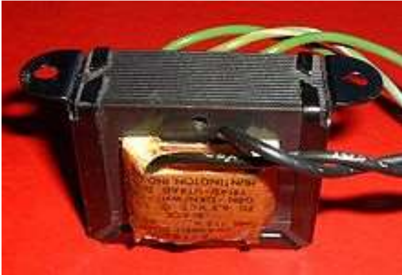
Laminated steel core transformer showing edge of laminations at top of photo
