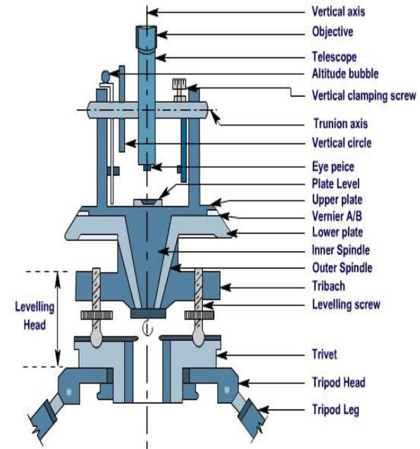
Figure 20.4 Sectional view of a Theodolite
