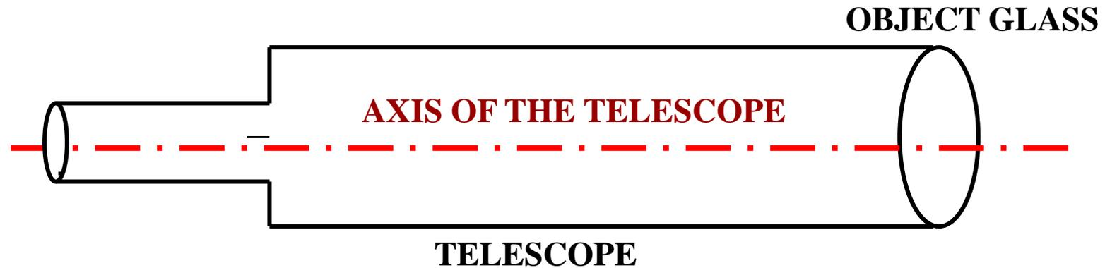
It is also known as an imaginary line joining the optical centre of the object-glass to the centre of eye piece.
