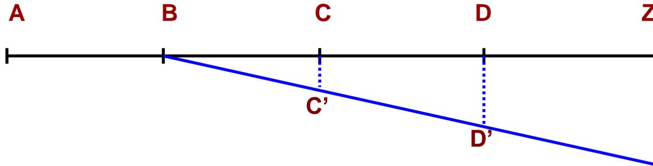
Now if the instrument is in adjustment, the points **A,B,C,D** and **Z** will be in one line, which is straight but if it is not in adjustment i.e. line of collimation is not perpendicular to the horizontal axis ,then **C', D'** and **Z'** will not be in a straight line.
