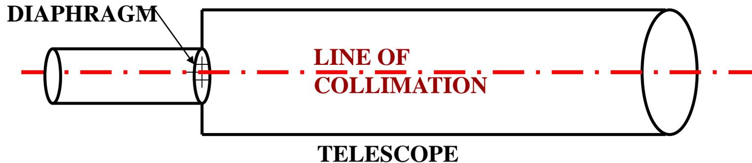
It is also known as the **line of sight**. It is an imaginary line joining the intersection of the cross-hairs of the diaphragm to the optical centre of the object-glass and its continuation.
