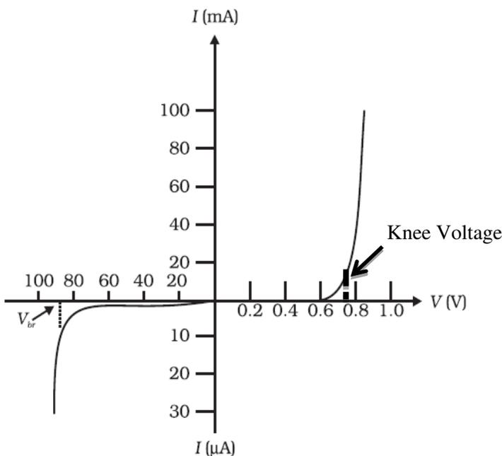
Let  $V$  is the voltage applied. This pushes the majority carriers, the holes in the p-type and electrons in the n-type towards the p-n junction.
