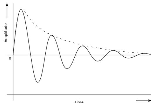
**Fig. 7.4.** Damped vibrations
