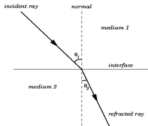
**Fig. 8.2** Refraction of light
