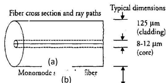
**Numerical Aperture (NA):** It is the light collecting ability of an optical fiber. It depends on difference in refractive index of core and cladding. Generally, value of NA ranges from 0.1 to 0.5 for most of the commonly used optical fibres.
