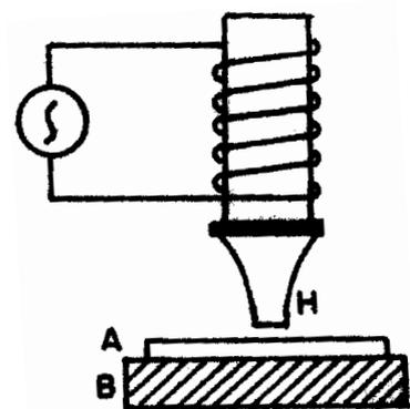
Fig. 7.7 Ultrasonic drilling
