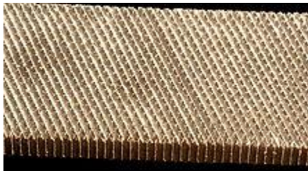
Detail of a double-cut flat file showing cutting surfaces milled on both wide and narrow faces
