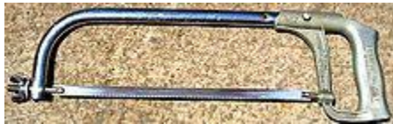
Typical full-size hacksaw frame, with 12" blade
